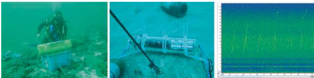
Fig. 12.14 Underwater acoustic recorders used to monitor the acoustic habitat of Cano and Murcielago Island in Costa Rica, both locations are protected areas used by humpback whales and dolphins. The last photograph shows spotted dolphin whistles recorder at 2 a.m. The project is funded and coordinated by Conservation International Costa Rica, and lead by Dr. May-Collado
